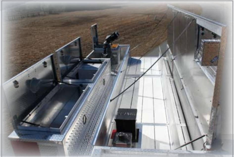
Roof top compartments extend into lower compartments for ground level access.
