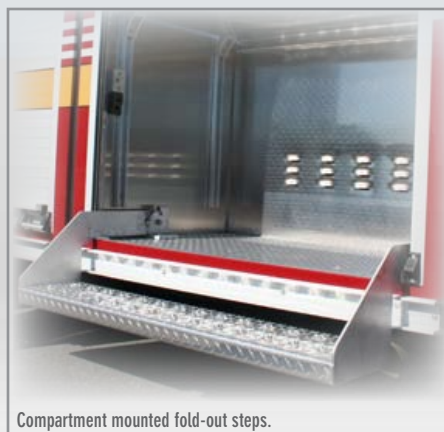
Compartment mounted fold-out steps.
